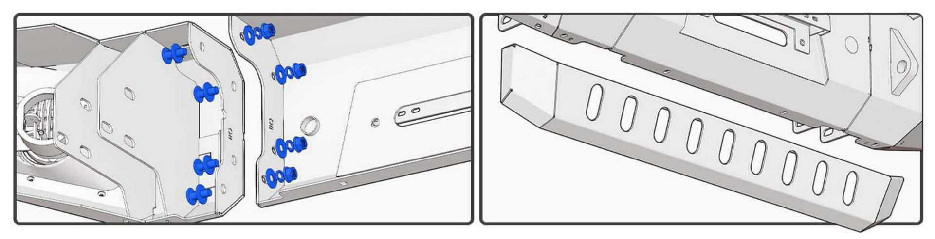
The bumper main body is assembled with four M10 screws, and after installation, the lower guard plate is secured with M8 screws.
