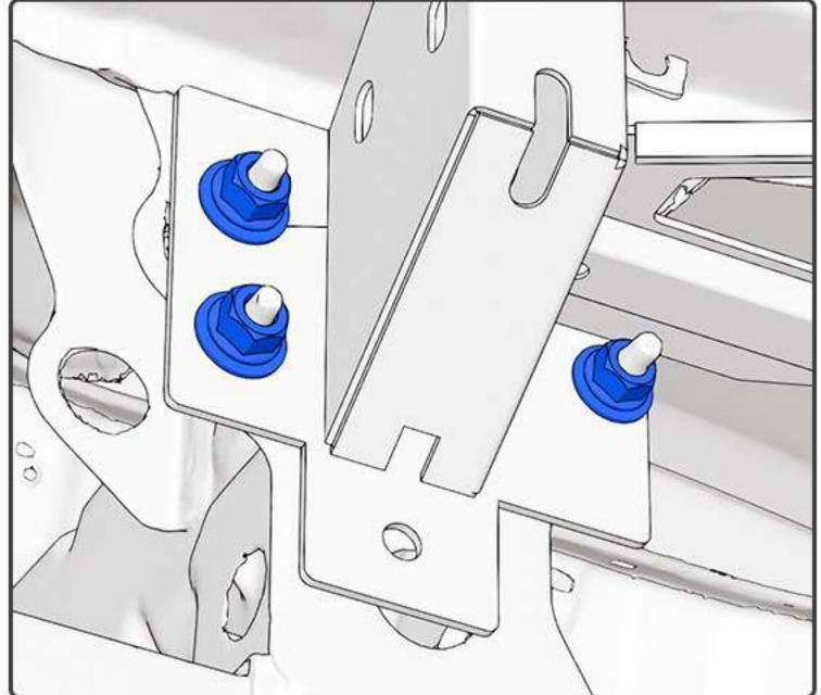
Locate and install the winch mounting bracket we provided. You can use the factory screws or the M12 nuts we supplied for fixing it.
