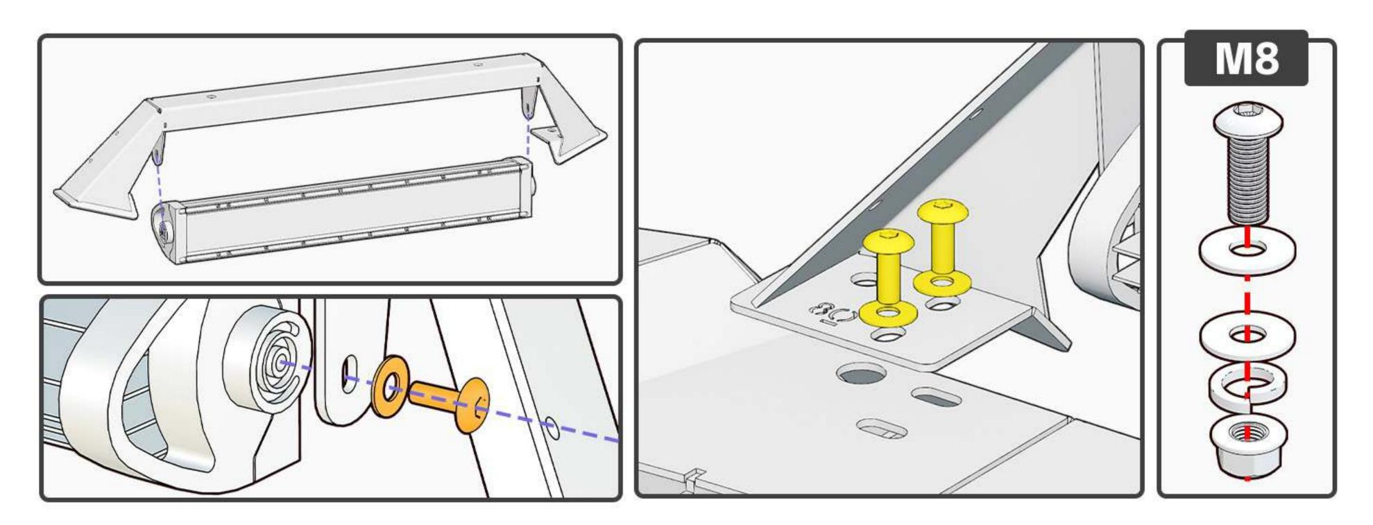
First, use M6 screws to assemble the strip light, then secure the lamp bracket with black M8 screws.
