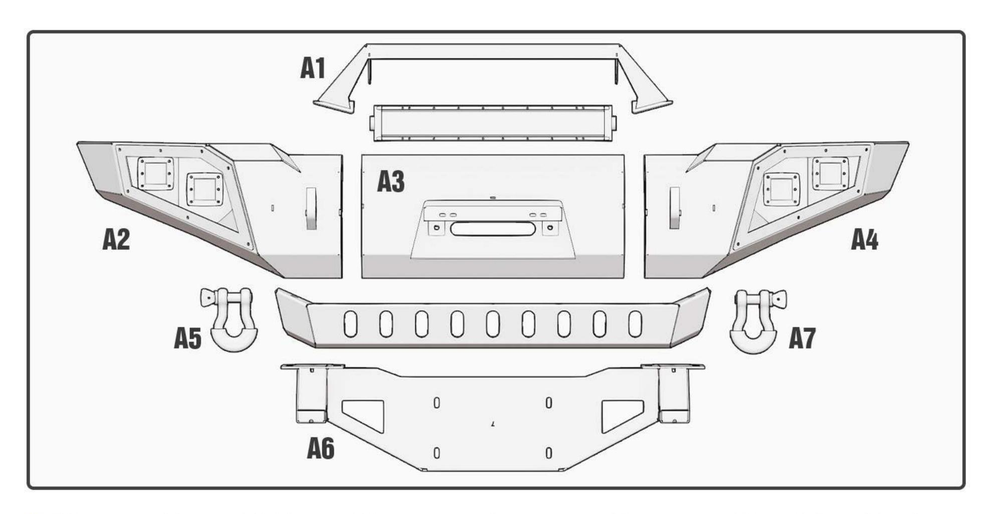
After unpacking and taking out the accessories, prepare the screws. Then, follow the steps to assemble the bumper completely.
