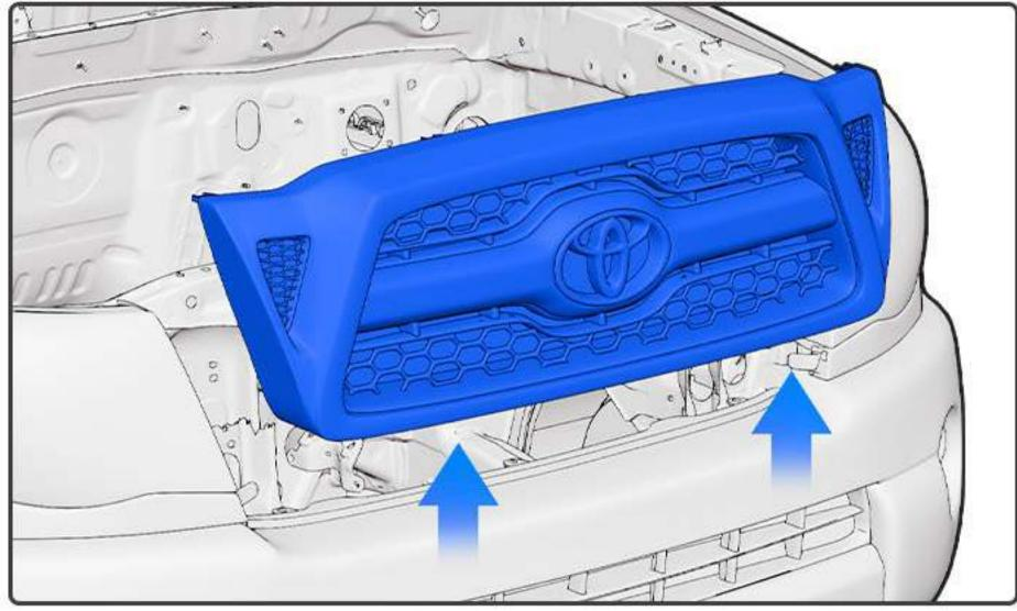
After opening the hood, remove the four fixing screws on the center grille and pull out the grille. Note that there are two plastic clips.
