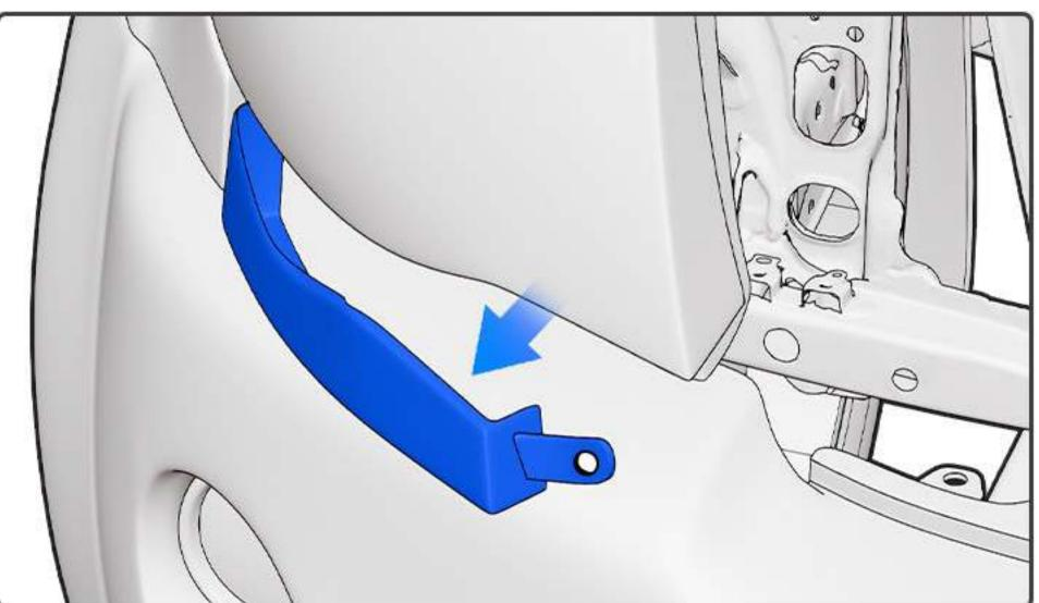
Locate the plastic part below the headlight, remove the screws, and then pull it out.
