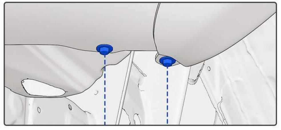
• Locate and remove the two screws from the inner lining. Then, use a ratchet wrench to remove the three screws on the top of the bumper. After that, find and remove the two fixing screws on the bottom of the bumper. Repeat the same steps on the other side.
