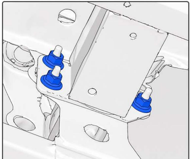
• Lift the bumper with your friend and remove it. Then, use a ratchet wrench to remove the three fixing screws of the front impact beam. Repeat the same steps on the other side.
