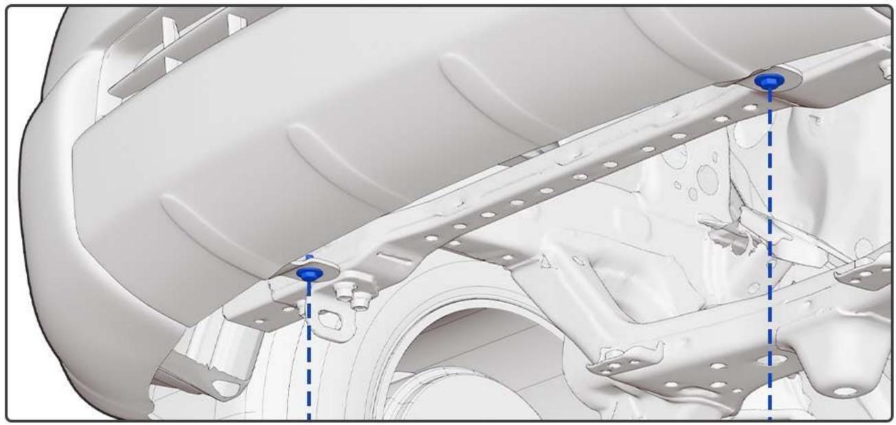
After flipping back the inner lining, locate and disconnect the wiring harness. Then, use a ratchet wrench to remove the two fixing screws at the bottom of the bumper.
